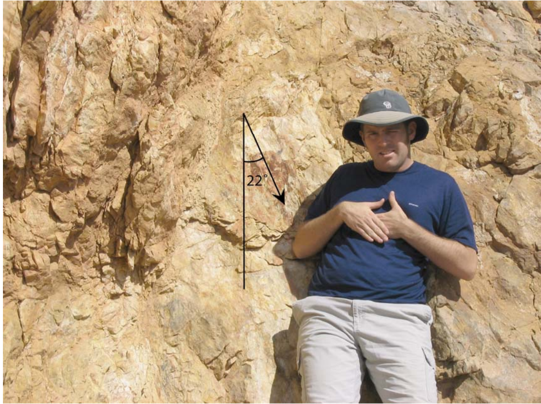
Figure 3. Slickensides demonstrating left-lateral movement along the hanging wall of the Teasdale Fault with a rake of 22^\circ . Photo taken at the point where Pleasant Creek intersects the Fault Trace.
